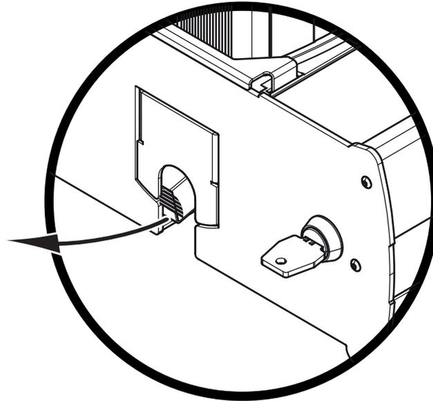
Evolis advises you to empty the reject hopper regularly, such as whenever the ribbon is changed or during routine maintenance. For the standard version (without central locking), it is sufficient just to remove the cards present in the reject hopper.
