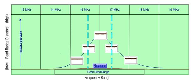
If cards are purchased with a resonant frequency of 14.0 MHz, the read range will drop to less than one inch. Purchasing cards and readers together, from the same manufacturer is critical. Guarantee peak performance by extensive testing conducted before introducing a new reader or card.
