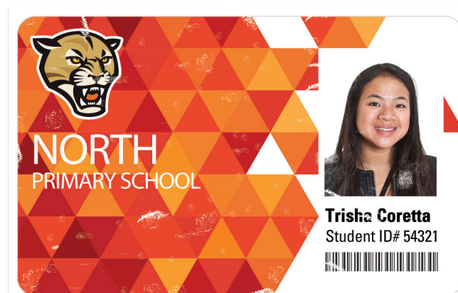
Card shows visible defects due to lack of routine printer maintenance
